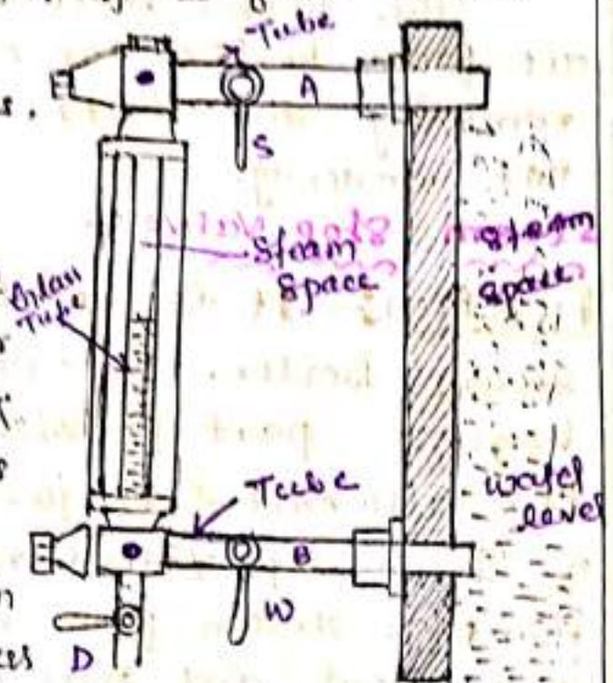
The rectangular passage at the ends of the glass tube certain two balls. In case the glass tube is broken, the balls are carried along its passage to the ends of glass tube and flow of water and steam out of the boiler is prevented.
