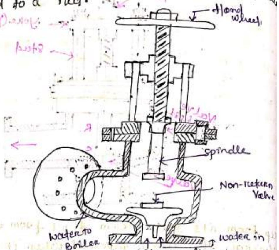
At normal working condition, the non-return valve is lifted due to the pressure of water from the pump and the water is fed to the boiler. But when the pump pressure falls below boiler pressure or if the pump stops, non return valve is closed automatically due to the pressure of the water from the boiler and prevents the escape of water from the boiler.
