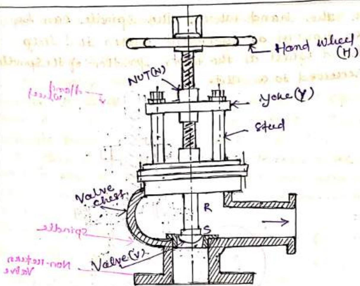
up from its seat, steam flows from the boiler through the steam pipe and when it is placed on its seat flow of steam from the boiler can no longer take place.
