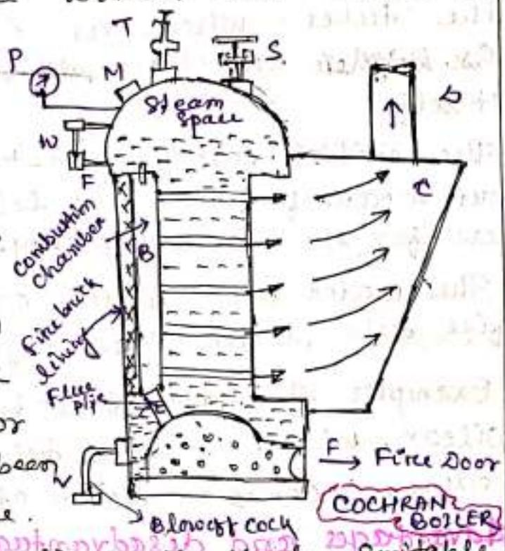
Cochran boiler is particularly suitable for its portability, the small amount of floor space required for its installation and the rapidity with which it can be put to work.
