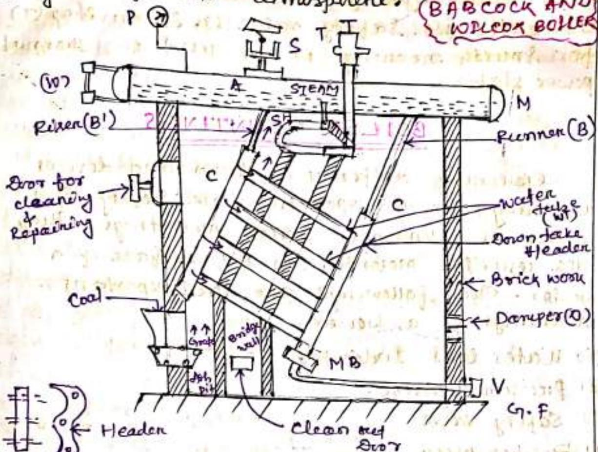
Due to continuous flow of flue gases surrounding the  $H_2O$  tubes. the circulating  $H_2O$  becomes more and more heated and ultimately it reaches its boiling point temp. and steam begins to be produced. The steam is passed through a superheater (SH) where it is further heated by the outgoing flue gases and thus it becomes superheated. The superheated steam is finally led out of the boiler through the steam stop valve (T).
